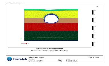
**Description:** Drainage tunnel, 40 m<sup>2</sup>cross-section-area, through rocks and soils, 2.7 km long tunnel
