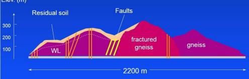
**Description:** Rock tunnelling through hard rock excavated by drilling and blasting, 96 m<sup>2</sup> cross-section and 1800 m long.
