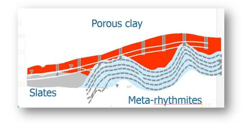
**Description:** Underground tunnel for the Brasília Underground (Metro) system, the shallow tunnel's section area is 80 m<sup>2</sup> and it is 6km long. It was excavated by conventional method (NATM)
