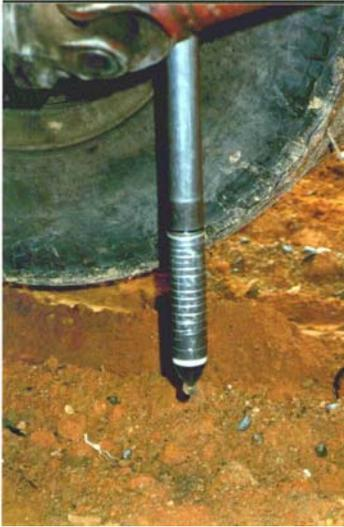
*Figure 20 Electronic cone just before insertion*
