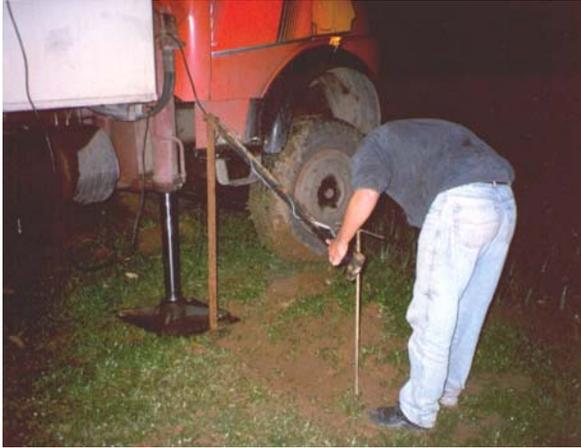
Figure 26 Details of hammer and strike plate for shear wave velocity measurements (with a CPT truck)
