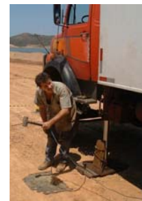
Figure 5 Generating shear waves at the ground surface
