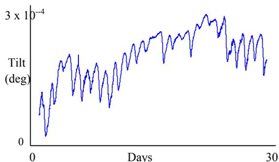
Figure 1. Tilt of a building over a one-month period
