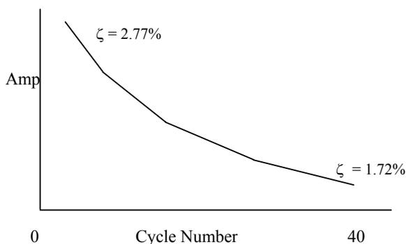
Figure 2. Extended decay of oscillation during an artificially induced shaking test
