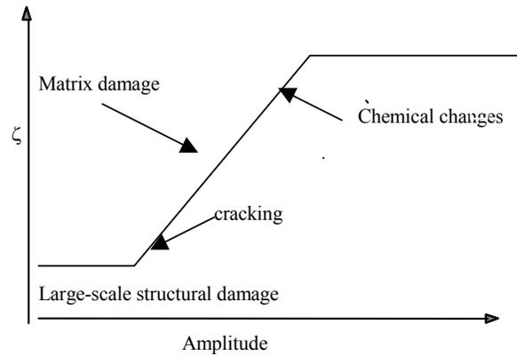
Figure 3. Non-Linear Damping Characteristic and the correlation with damage
