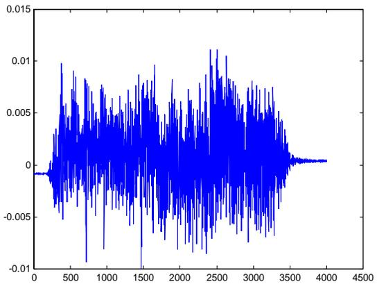
Fig 6: Horizontal response measured on the trelice
