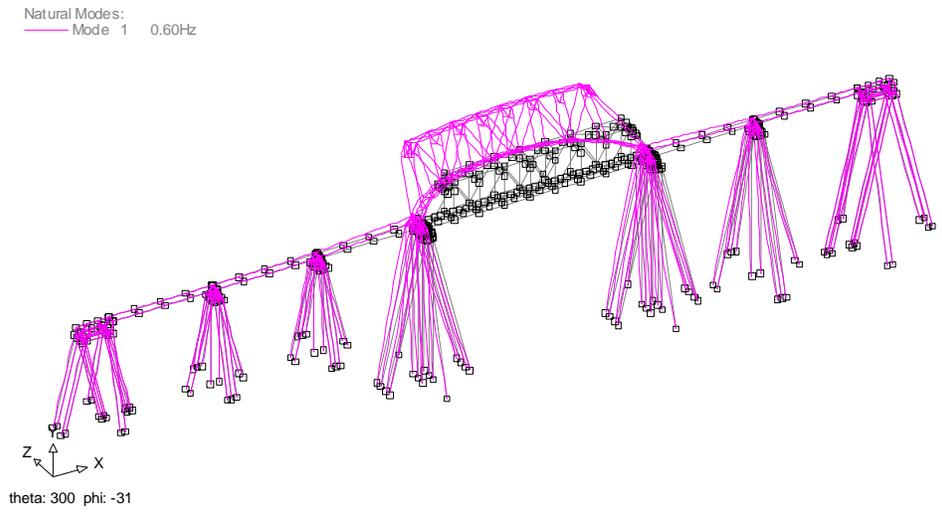
Fig 5: First mode of the model with damage introduced (0.60Hz.)
