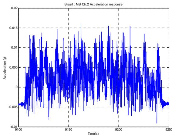
Fig 2: Vertical acceleration response of the bridge
