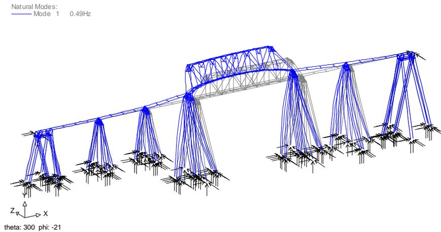
Fig 4: First mode of the undamaged model (0.49 Hz.)
