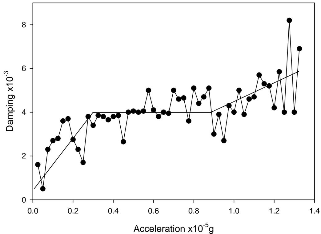
Fig. 8: Horizontal damping characteristic for the bridge
