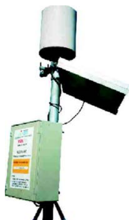
Figure 2. The automatic raingauge.
