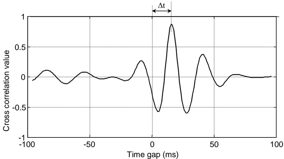
**Figure 7 Typical cross correlation function of two seismic signals**
