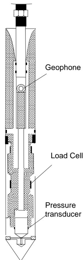
**Figure 1** Seismic piezocone
