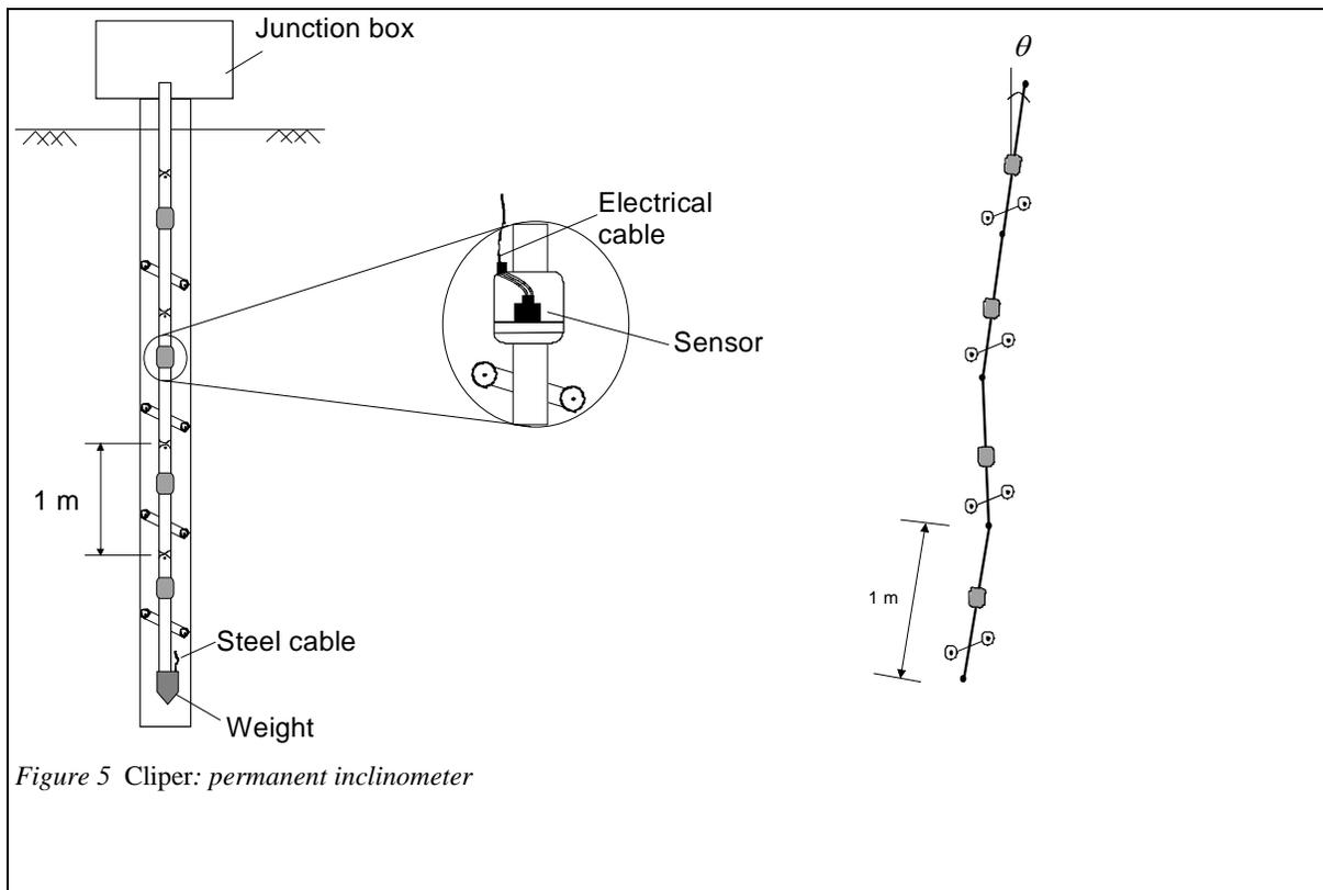
Figure 5 Cliper: permanent inclinometer
