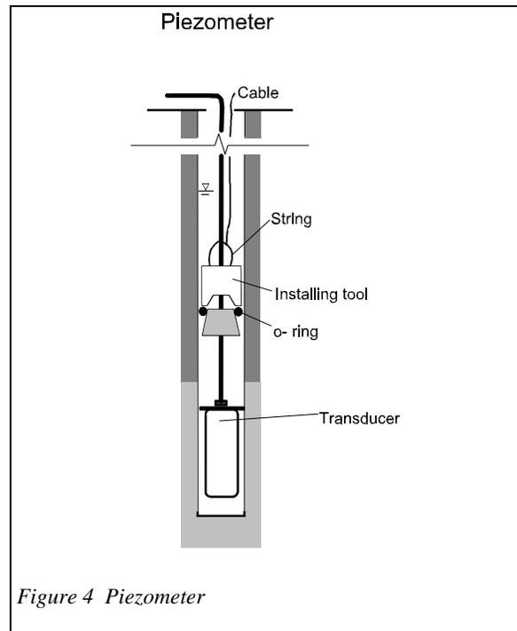
Figure 4 Piezometer
