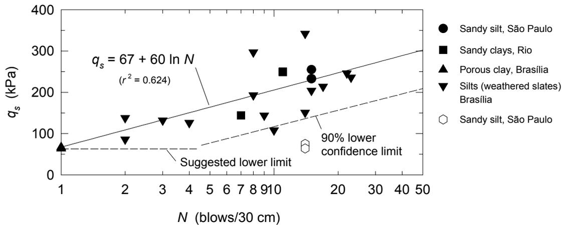
Figure 1 Pull -out tests results
