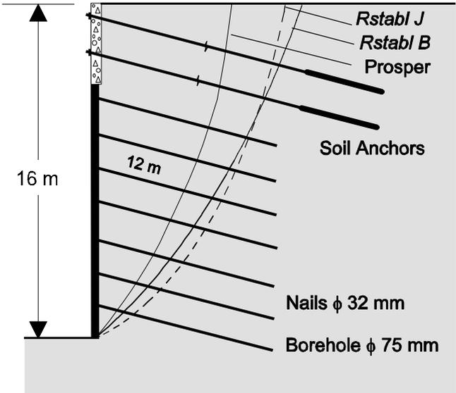
Figure 3 Mixed soil nailing structure proposed for an excavation in medium sandy-silt
