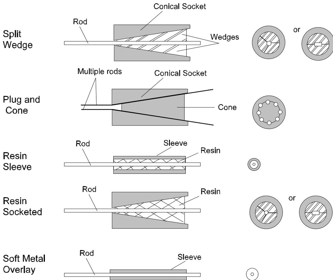
Figure 7 - Anchor head designs (Holte et al, 1994)
