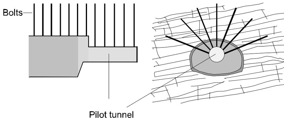
Figure 9 Rock bolting from a pilot tunnel
