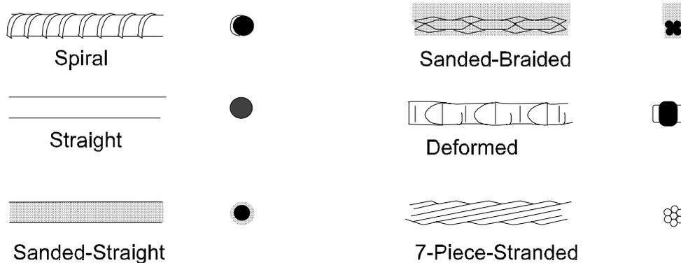
Figure 6 Types of surface finishing (Yamasaki et al, 1994)
