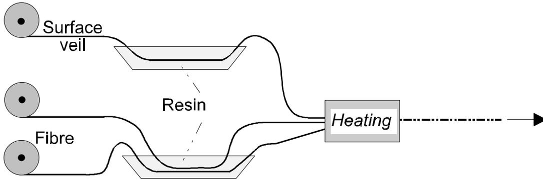
Figure 2 Pultrusion process
