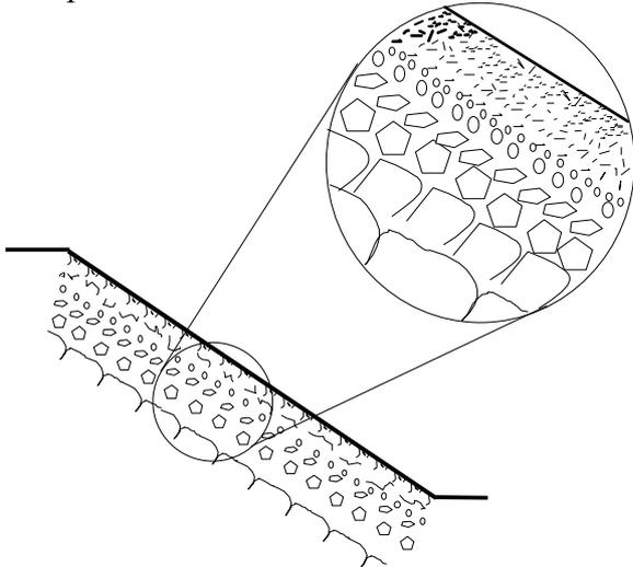
Figure 1 Slaking of the Tertiary clay crust due to swelling
