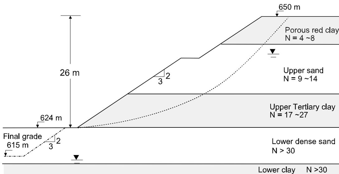
Figure 2 Failure in a 26 m high slope (initial design)
