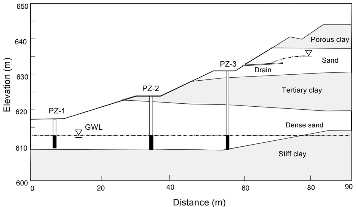
Figure 8 Ground water level in the sand layers
