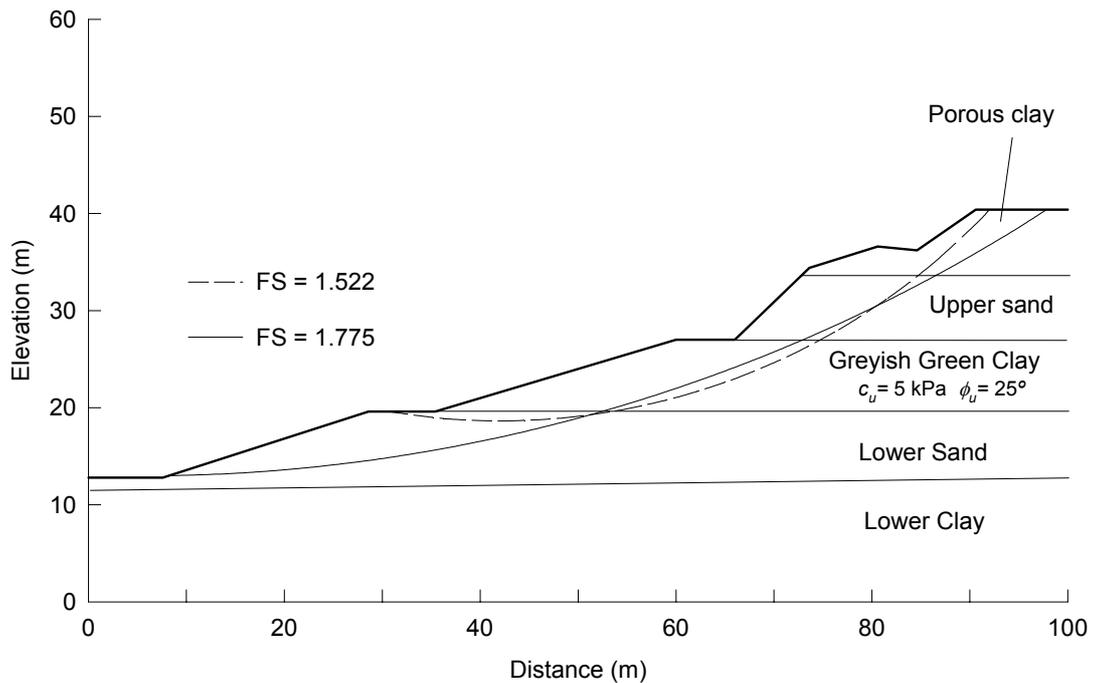
Figure 10 Stability analysis for the final design
