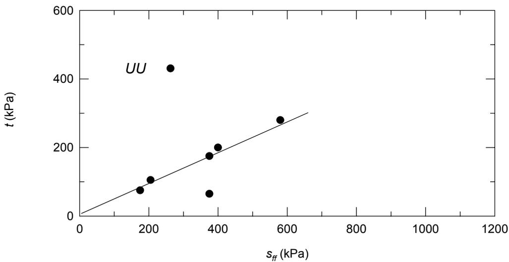
Figure 4 UU tests in the greyish green Tertiary clay
