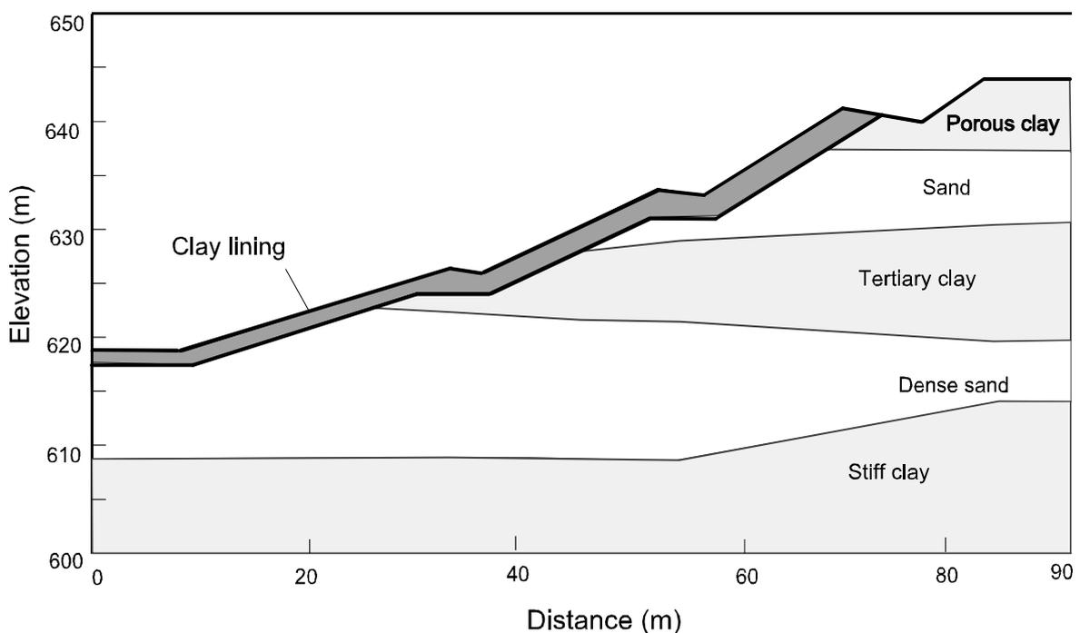
Figure 11 Final cross section design
