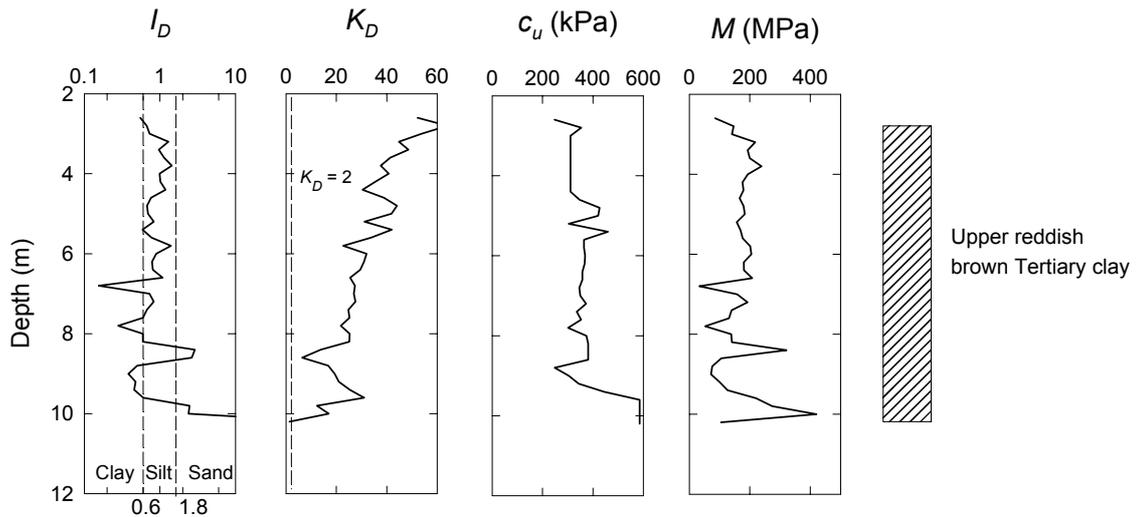
Figure 5 DMT profile in the upper reddish brown Tertiary clay
