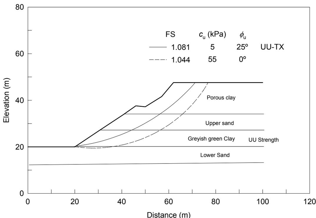
Figure 9 Back-analysis of the major failure
