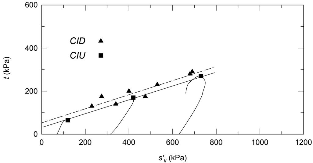
Figure 3 Triaxial tests in the Tertiary clay
