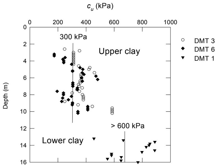
Figure 7 Shear strength from the DMT at the upper and lower Tertiary clay layers
