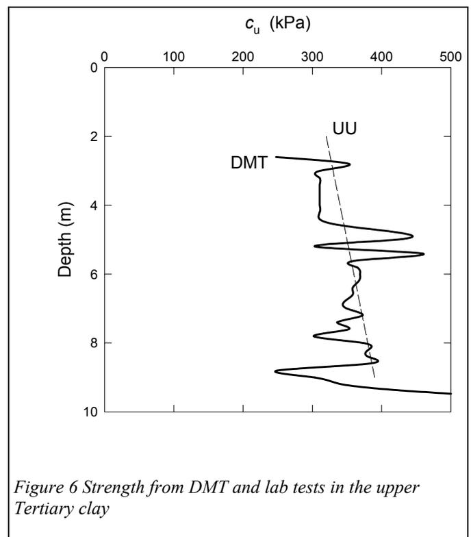
Figure 6 Strength from DMT and lab tests in the upper Tertiary clay
