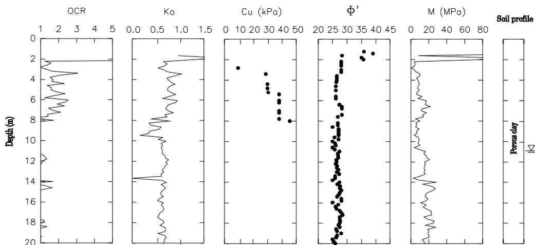
Figure 8 Typical results from DMT test (SP608)
