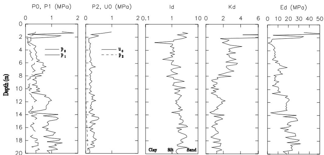
Figure 7 Typical results from DMT test (SP608)
