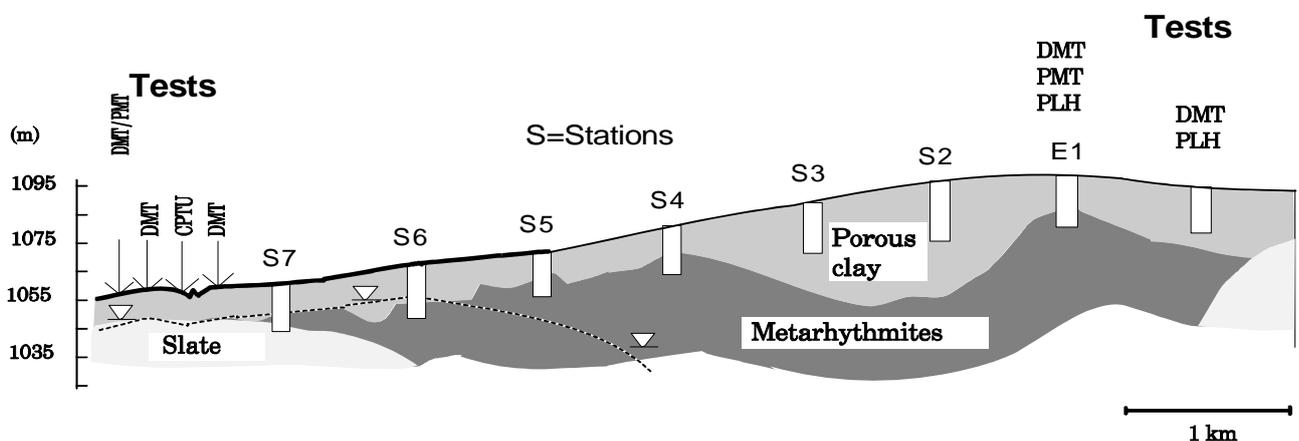
Figure 4 Soil profile along the tunnel, South Wing, Brasília
