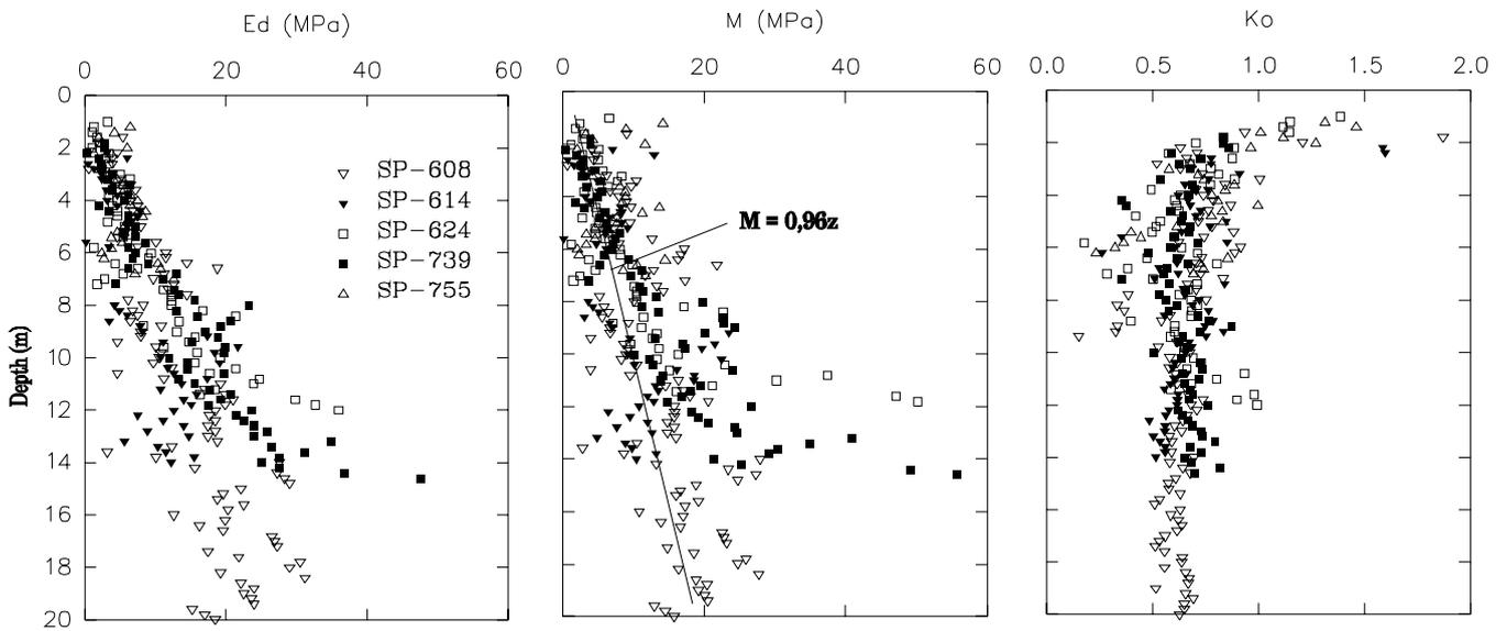
Figure 9 Deformation moduli and  $K_0$  from several DMT's in the porous clay
