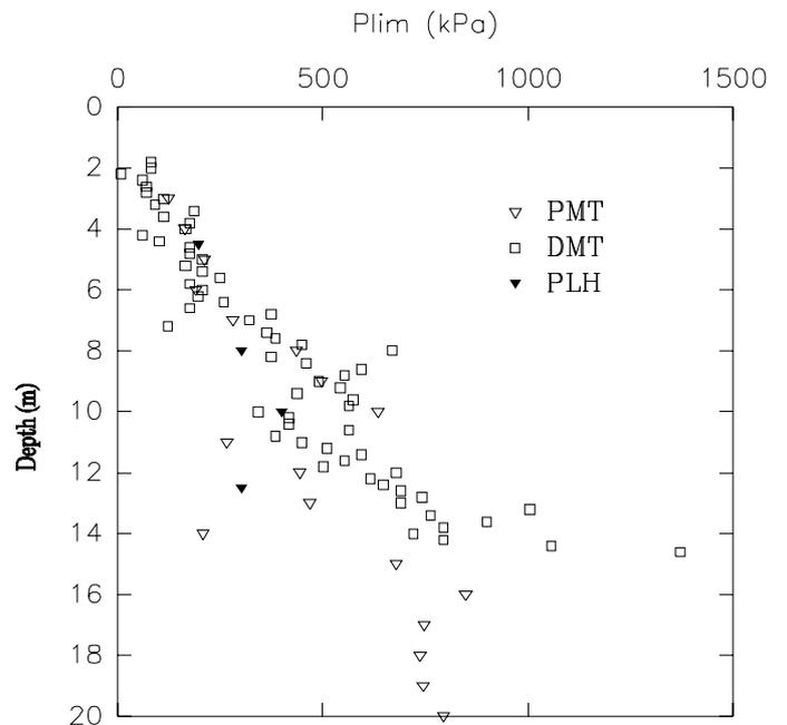
Figure 11 Limit pressure  $p_{lim}$  from PMT, DMT and PLH
