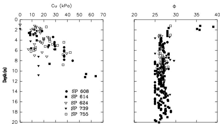
Figure 10 Strength parameters from DMT in the porous clay
