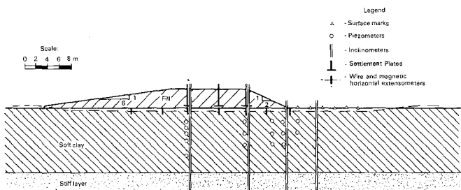
FIG. 5.—Main Section—Instrumentation Scheme
